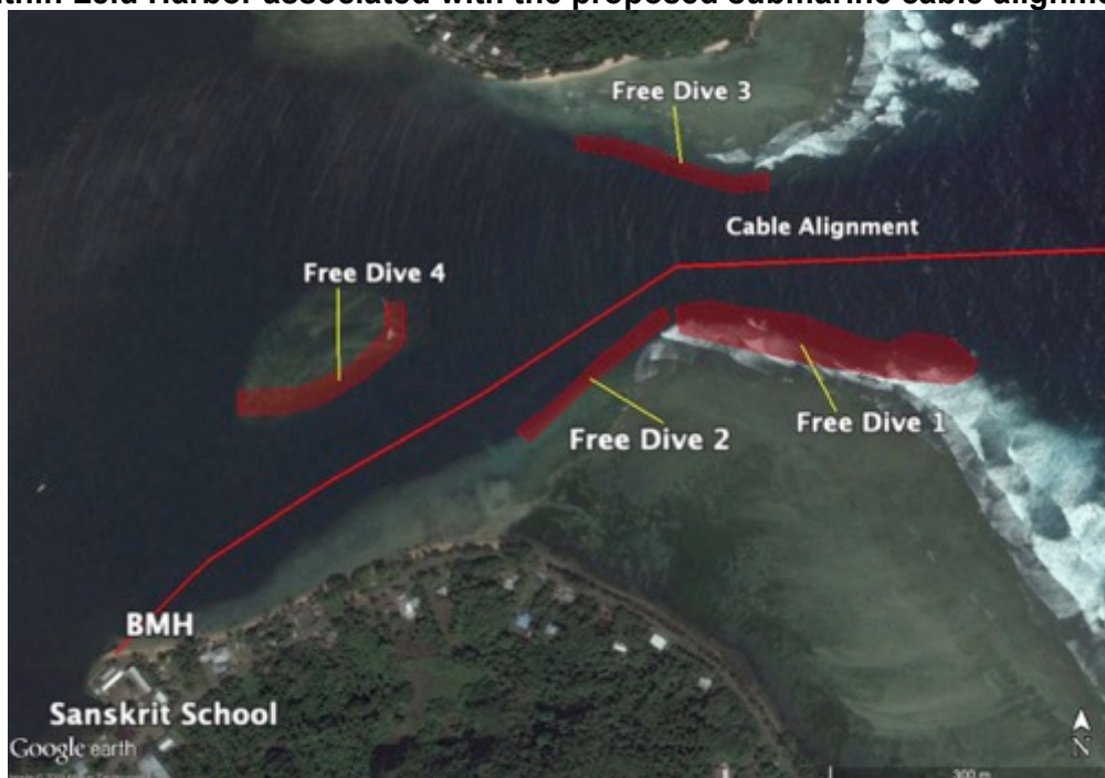
Figure 7: Location of the four Free Dive benthic marine assessment sites within Lelu Harbor associated with the proposed submarine cable alignment.
